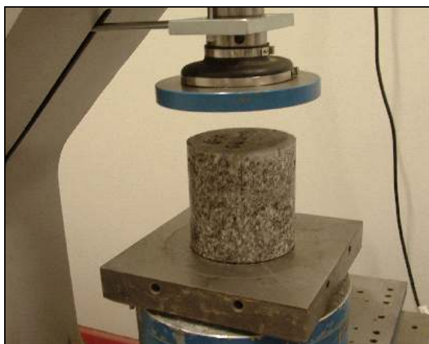
Figure 6: Compressive strength testing of a 1:1 height to diameter specimen of HBM
