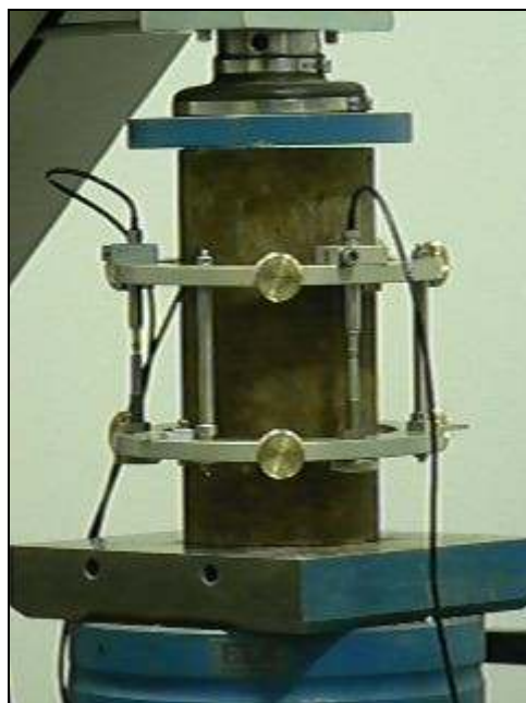
Figure 7: Strain collar fitted to a 2:1 HBM specimen during modulus of elasticity testing
