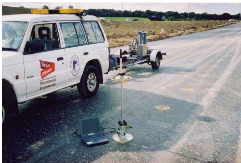
Figure 10: LWD testing being carried out on a pavement to assess the surface modulus
